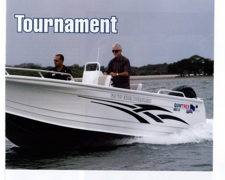
Design: The new 610 Top Ender is quite an impressive package on the trailer, measuring some 6.1m in total including the bowsprit roller and maxipod M3 transom. Beam is 2.4m and the hull depth a generous 140cm.
